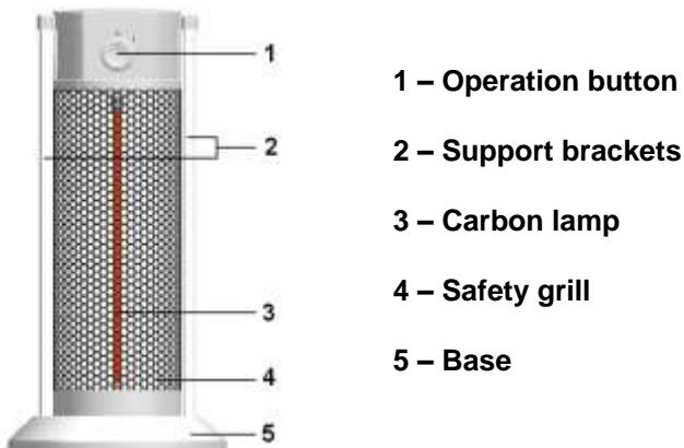
The heater is fitted with a **tipping safeguard** which automatically shuts off the appliance if it inadvertently falls over. When the heater is returned to its upright position, it will resume functioning as normal but, before reusing, switch off, unplug and check for damage. Do not use the heater if it is damaged or malfunctioning, but have it inspected/repaired!
